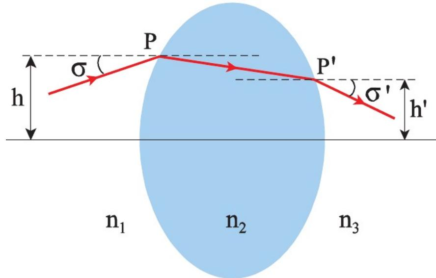
$$\begin{bmatrix} h' \\ \sigma' \end{bmatrix} = [R_{P'}][T_{PP'}][R_P] \begin{bmatrix} h \\ \sigma \end{bmatrix} = [L] \begin{bmatrix} h \\ \sigma \end{bmatrix}$$
