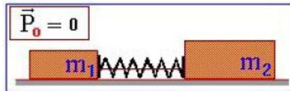
$$\vec{P}_f = \vec{P}_0 \quad \therefore \quad m_1 \vec{v}_1 + m_2 \vec{v}_2 = 0 \quad \therefore \quad \vec{v}_1 = -\frac{m_2}{m_1} \vec{v}_2$$
