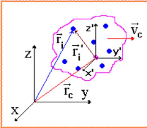
$$\begin{aligned}\vec{r}_i &= \vec{r}_c + \vec{r}'_i \\ \vec{v}_i &= \vec{v}_c + \vec{v}'_i \\ \vec{a}_i &= \vec{a}_c + \vec{a}'_i\end{aligned}$$
