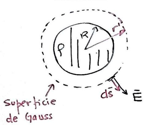
$$\begin{aligned} \Phi_{\vec{E}} &= \oint_S \vec{E} \cdot d\vec{s} \\ &= \int_0^{2\pi} \int_0^\pi E r^2 \sin\theta \, d\theta \, d\phi \\ &= E r^2 4\pi = \frac{q_{\text{enc}}}{\epsilon_0} \end{aligned}$$
