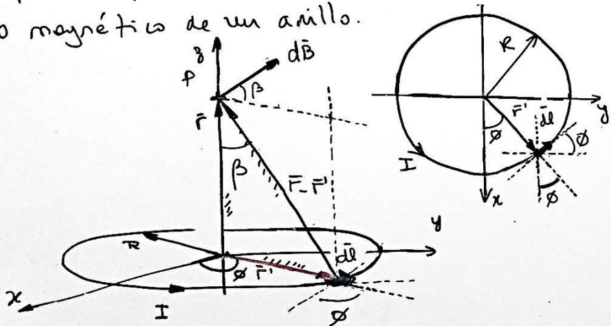
$$d\vec{B}(P) = \frac{\mu_0 I}{4\pi} \frac{d\vec{l} \times (\vec{r} - \vec{r}')}{|\vec{r} - \vec{r}'|^3} \quad \hat{e}_{\vec{r}-\vec{r}'} = \frac{\vec{r} - \vec{r}'}{|\vec{r} - \vec{r}'|}$$
