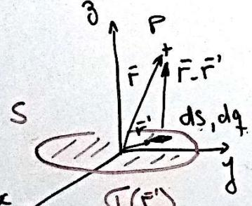
Diagram showing a plane  $S$  in a 3D coordinate system ( $x$ ,  $y$ ,  $z$  axes). A small element  $dS$  is shown at position  $\vec{r}'$  with a surface charge density  $\sigma(\vec{r}')$ . The vector from the origin to the element is  $\vec{r} - \vec{r}'$ .
