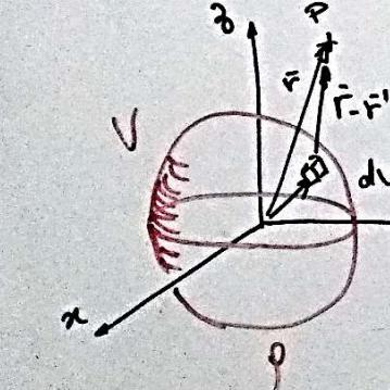
Diagram showing a volume  $V$  in a 3D coordinate system ( $x$ ,  $y$ ,  $z$  axes). A small element  $dV$  is shown at position  $\vec{r}'$  with a volumetric charge density  $\rho(\vec{r}')$ . The vector from the origin to the element is  $\vec{r} - \vec{r}'$ .
