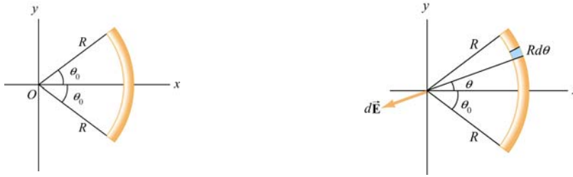
Figure 2.13.2 (a) Geometry of charged source. (b) Charge element dq
