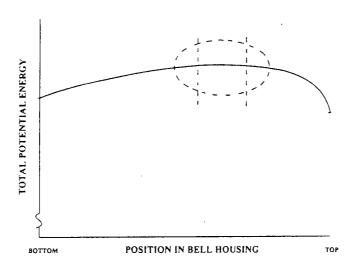
Everyday observation shows that things tend to move to a place of lower potential energy. Imagine that the plastic plates have been removed. Without the ceramic magnets, the cube would fall to the lowest place it could get. The first graph shows that this is the place with the lowest potential energy.
