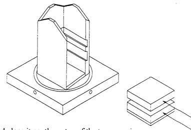
Hold the small cube-shaped magnet, and place it gently on top of the top ceramic magnet at the top of the apparatus. When you release it, it will rotate if needed so that it is attracted by the ceramic magnet. DON'T let it fly toward the ceramic magnet. It is both expensive and brittle.
